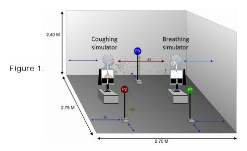
NIOSH aerosol samplers collect air from the mouth and at various positions (P1,P2,P3) within the room. All inside dimensions in centimers.
