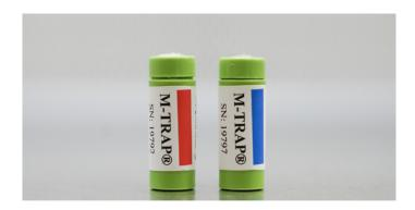
The M-TRAP® is a unique air sampling cassette developed specifically for the rapid capture and analysis of airborne fungi, bacteria, and viruses using state-of-the-art DNA & RNA analysis. The M-TRAP® embodies the next generation of capture technology for residential and occupational mold exposure assessment. It excels where spore traps and agar impactions fall short: spore capture efficiency and turnaround time. Example analyses are: **SIAM** (Survey of Indoor Airborne Molds) or **Total Fungi**.
